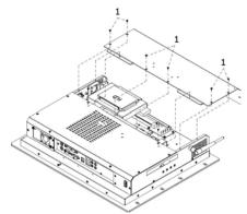
2. Remove the HDD form rear cover.
