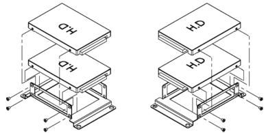
3. Please attach the HDD to rear cover and fasten screws.
